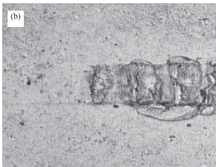
Figure 3 : Swinging module data for a TiN coating (thickness = 1 \mu\text{m} ) on a 440C steel substrate. The sudden jump in both the AE and Ft signals in the MST data (a) can be directly correlated to the coating failure shown in the optical micrograph (b).
