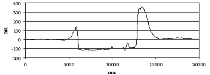
**Figure 2** : SFM cross-sectional profile through the image shown in Fig.1 (b). The depth at which coating failure occurs can be accurately measured as being 100 nm below the surface. This corresponds to the interface between the substrate and first coating.
