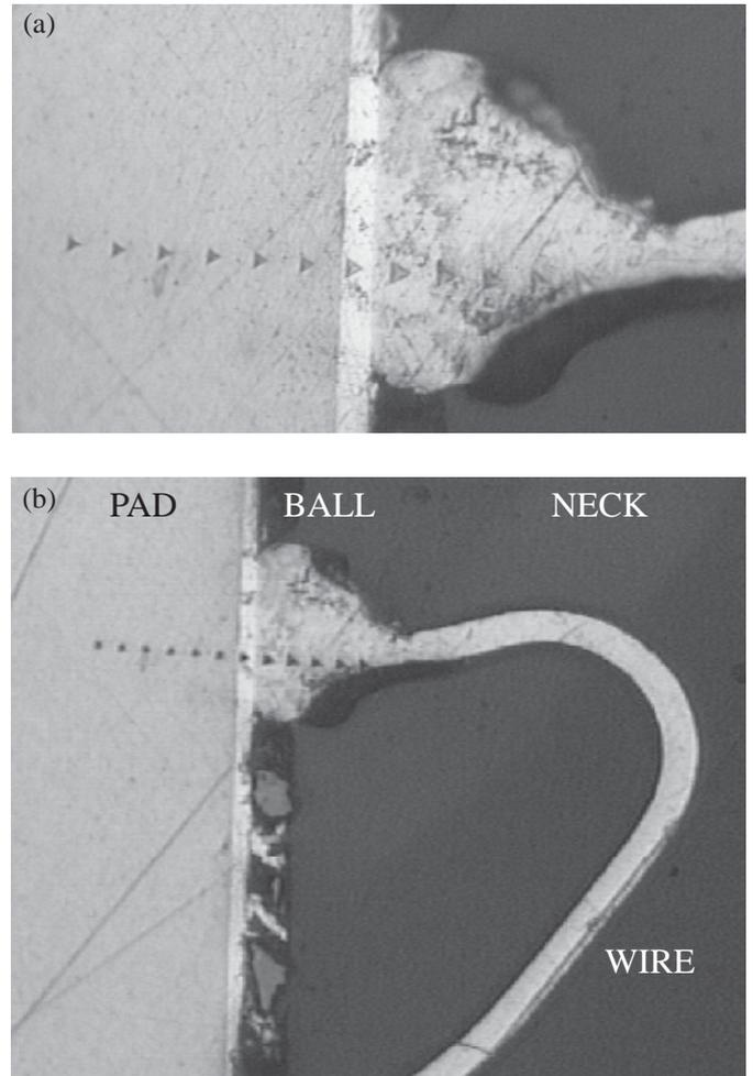
**Figure 1 :** Optical micrographs of a typical sectioned sample on which a line of 12 nanoindentations have been made. The overview (b) shows the different areas of the sample which can be compared, whereas the close-up (a) shows the positioning accuracy of the NHT in locating an indent on the silver coating which acts as an interface between the gold wire ball and the copper substrate.
