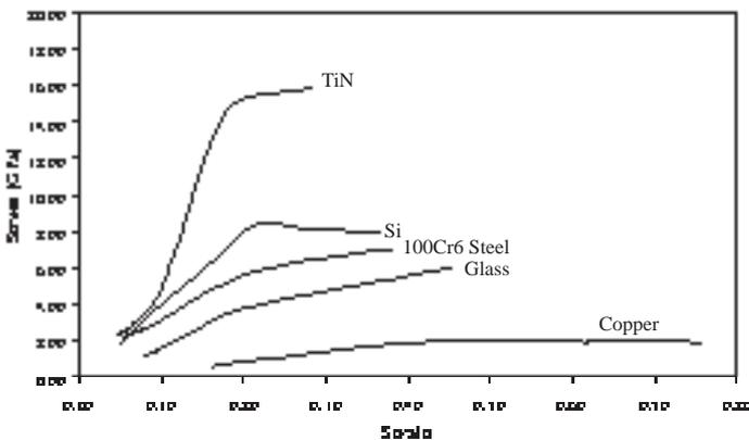
**Figure 1** : Stress-Strain data for TiN (coating thickness = 3  $\mu\text{m}$ ), pure Si, 100Cr6 steel, glass and pure copper calculated from multicycle indentations performed over the range 10 - 260 mN with a spherical indenter of radius 1  $\mu\text{m}$ . Each data set corresponds to the average of five sets of measurements.
