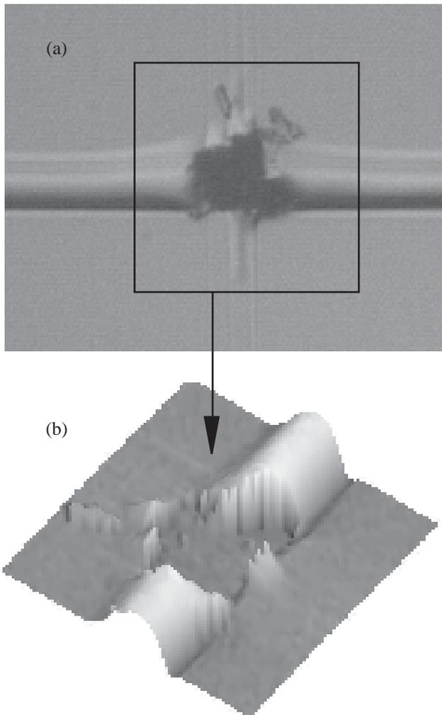
**Figure 1** : Result of transversal scratches on a typical damage area having undergone 70 cycles with an applied load of 2 mN and spherical indenter of radius 2  $\mu\text{m}$ . The optical micrograph (a) clearly shows the resulting decohesion and the SFM image (b) confirms the depth at which failure has occurred.
