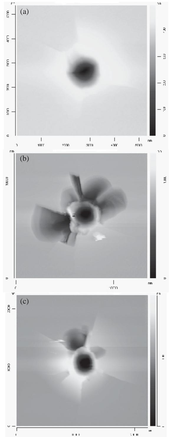
**Figure 2** : SFM images of residual monocyte indentations performed in Si with maximum applied loads of (a) 30 mN, (b) 100 mN and (c) 200 mN. The indenter was a spherical diamond of radius 1  $\mu\text{m}$ . Cracking becomes apparent even at low loads with severe chipping occurring at higher loads.
