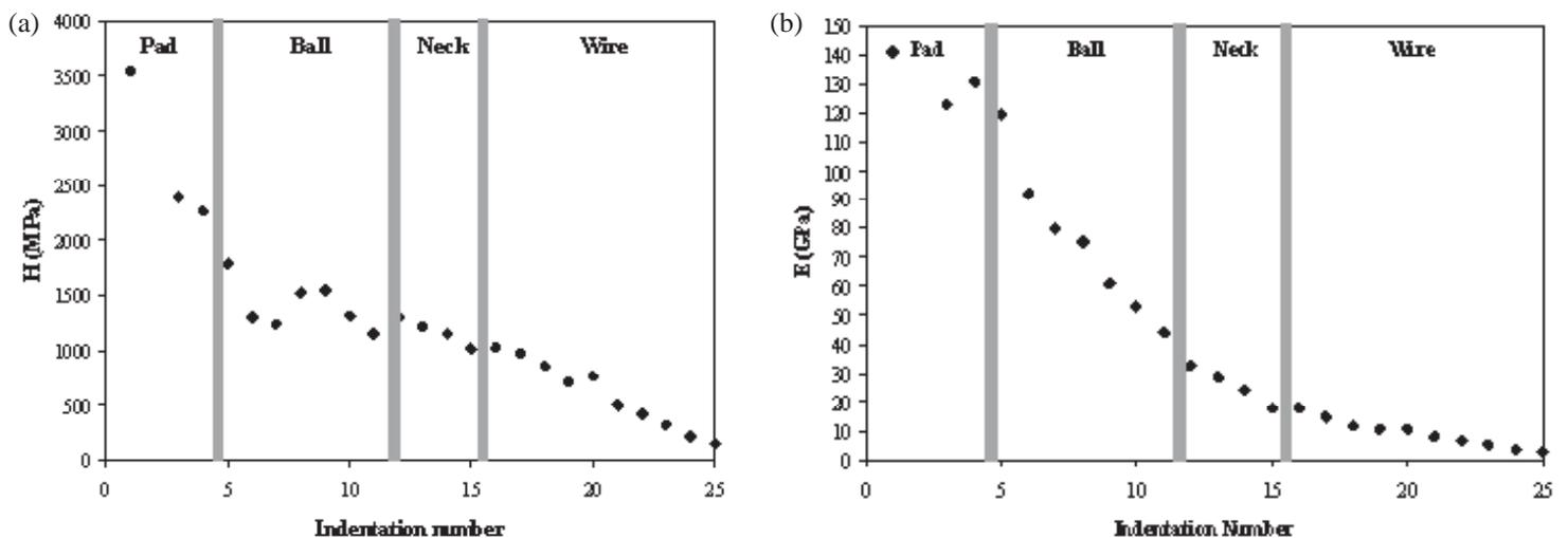
**Figure 2 :** Hardness (a) and Elastic Modulus (b) values plotted as a function of distance over the different tested areas of the gold wire bonded sample. Test conditions were 10 mN maximum load, 20 mN/min. loading rate and the indenter was of Berkovich geometry.
