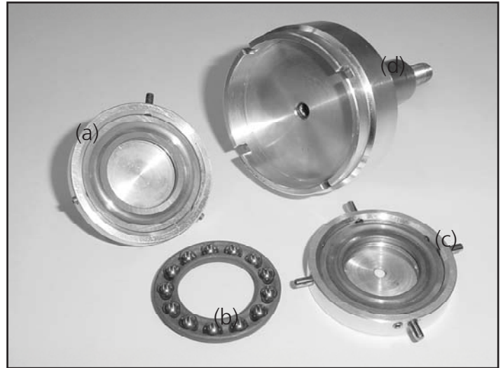
Figure 2 : The component parts of a single row bearing: upper casing (a), inner bearing (b), and lower casing (c) which is located in a specially modified sample support shaft (d).
