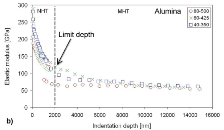
**Fig. 2** – Hardness (a) and elastic modulus (b) as a function of indentation depth measured on cross-section of alumina coatings. For clarity reasons the error bars were omitted.
